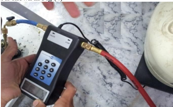
Fig(3) Electronic Refrigerant Charging Scale connected with refrigerant cylinder and refrigerator
